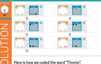
Here is how we coded the word "Thymio". You have to pass your finger on each sensor in the correct order to hear the entire sequence. Try to program Thymio to provide Morse code for other words.
