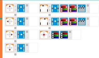
If you program one line for the left ground sensor and one for the right, Thymio will react if it senses something on the left or on the right. With only one block and two black sensors, Thymio should completely cross the black line before lighting up and making noise!
