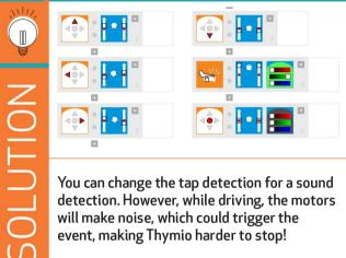
You can change the tap detection for a sound detection. However, while driving, the motors will make noise, which could trigger the event, making Thymio harder to stop!
